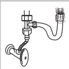
Connect supplied T valve to the toilet fill valve. Note T valve will be connected directly to toilet fill valve, not the shut off valve. Then connect rest of water lines to connected T valve.
