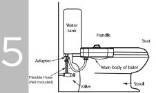
Open shut off valve and check for any leaks.
